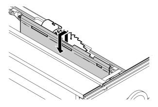
6. To block the saw blade insert lock bar into hole in the saw table and turn saw blade by hand until lock bar engages in saw spindle hole.
